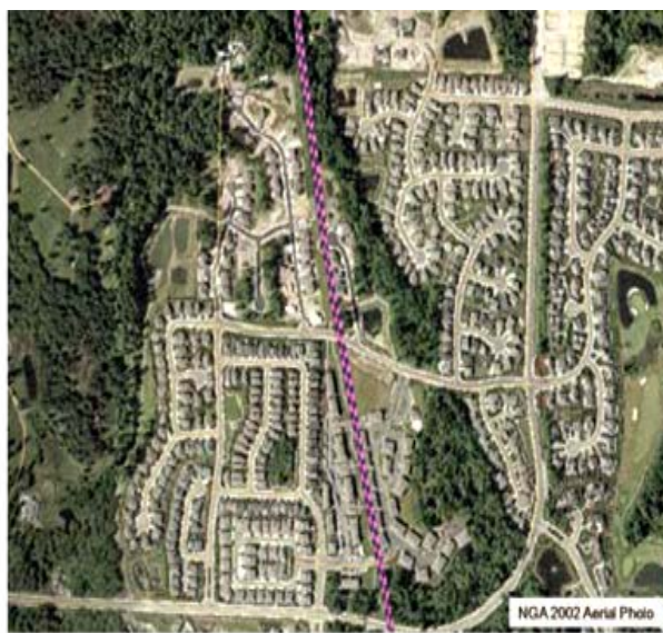
Figure 1: Development near a Transmission Pipeline in Washington State 1990-2002 (Sources: U.S. Geological Survey (left) and National Geospatial Intelligence Agency (right)) (U.S. GAO Report, GAO-12-388, Pipeline Safety, March 2012)
